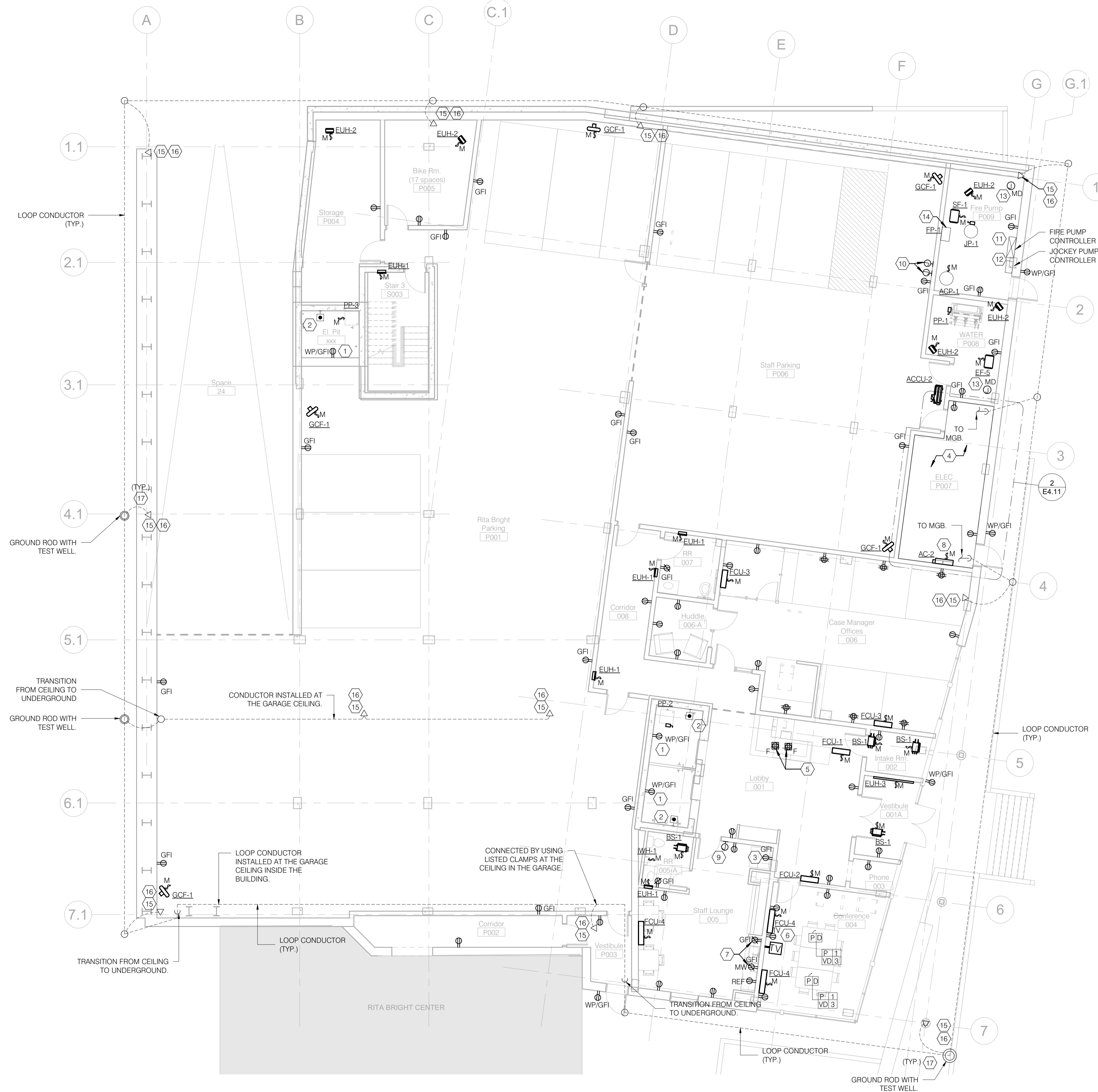
1 PARKING LEVEL PLAN - ELECTRICAL POWER 1/8" = 1'-0"
